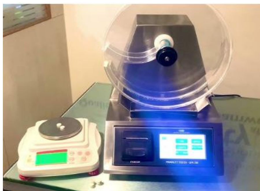
Figure 8: Friability Check with the Roche Friabilator
