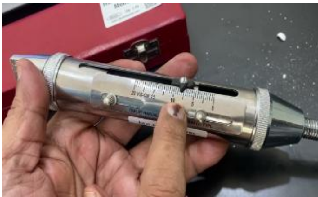
Figure 6: Monsanto Hardness Tester Testing for Hardness
